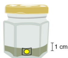
Figure 5.7. Glass jar used in the set-up based on the use of oxygen scavenger.
