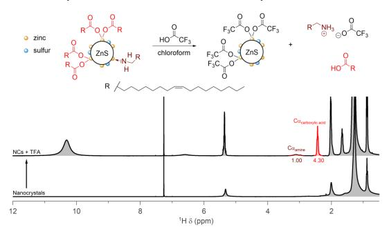
**Figure S5.** Surface chemistry analysis by means of ligand stripping by making use of a strong acid, i.e., trifluoroacetic acid (TFA), characterized by quantitative <sup>1</sup>H NMR (ERETIC). The purified NCs surface is identified with an 81%/19% mixture of oleate/oleylamine respectively.
