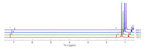
**Figure S1.** Pure poly(ODE) is obtained by heating at temperatures between 120 and 320°C for 24 hours and standard purification. <sup>1</sup>H NMR analysis in CDCl<sub>3</sub> (\*) indicates the removal of the terminal alkene group of ODE at 5.80 an 4.94 ppm. Residual solvent peaks may occur of water (α) at 1.5 ppm.<sup>8</sup>
