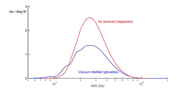
**Figure S2.** Size exclusion chromatography of poly(ODE) formed at 240 °C for 24 hours from 1-octadecene which is used after vacuum distillation and as-received after degassing (for 1 hour at 40 °C, repeated 3 times).
