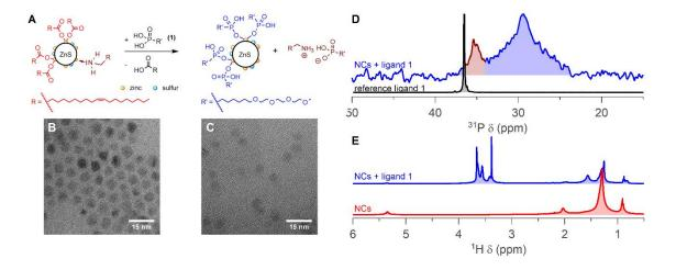
**Figure S6.** (A) Scheme of rational ligand exchange reaction of 81% oleate and 19% oleylamine capped surface of ZnS:Mn/ZnS NCs with ligand **1**. (B) TEM image of ZnS:Mn/ZnS NCs, stabilized with oleate and oleylamine, deposited from chloroform. (C) TEM image of
