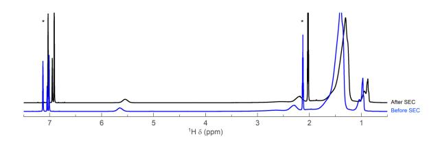
**Figure S4.** Purification of oleate stabilized NCs from poly(ODE) in a mixture by means of size exclusion chromatography (SEC) is unsuccessful. After SEC, <sup>1</sup>H NMR still shows a double peak at the methyl region (1 ppm) comparable to before.
