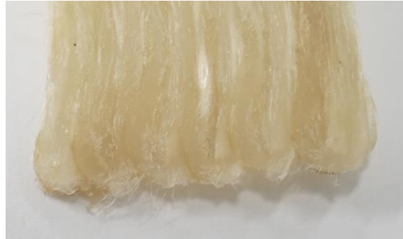
Figure 3. Tow pullup in regions of high path curvature.
