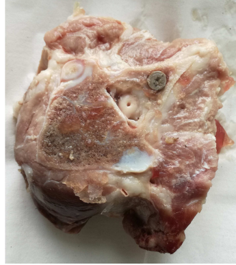
Figure 5.3: Beef vertebra with PMMA-MNP sample (grey)
