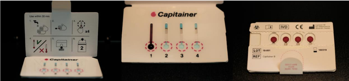
Figure 3 The Capitainer-B device. Picture 1 (left) showing the inside of the device containing user instructions; Picture 2 (middle) demonstrating the application of a drop of blood at the inlet port; Picture 3 (right) displaying 4 filled pre-perforated paper discs.
