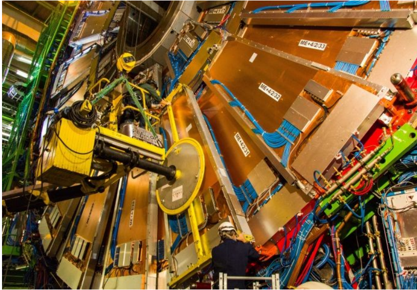
Figure 4.2: The Cathode Strip Chamber region in the CMS muon system.
