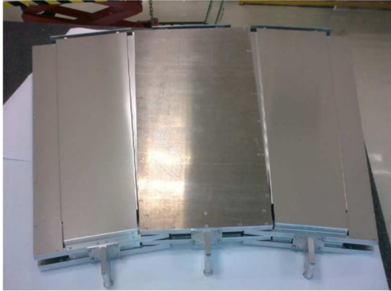
Figure 5.46: GE1/1 Superchamber dummy design version with short and long chambers.
