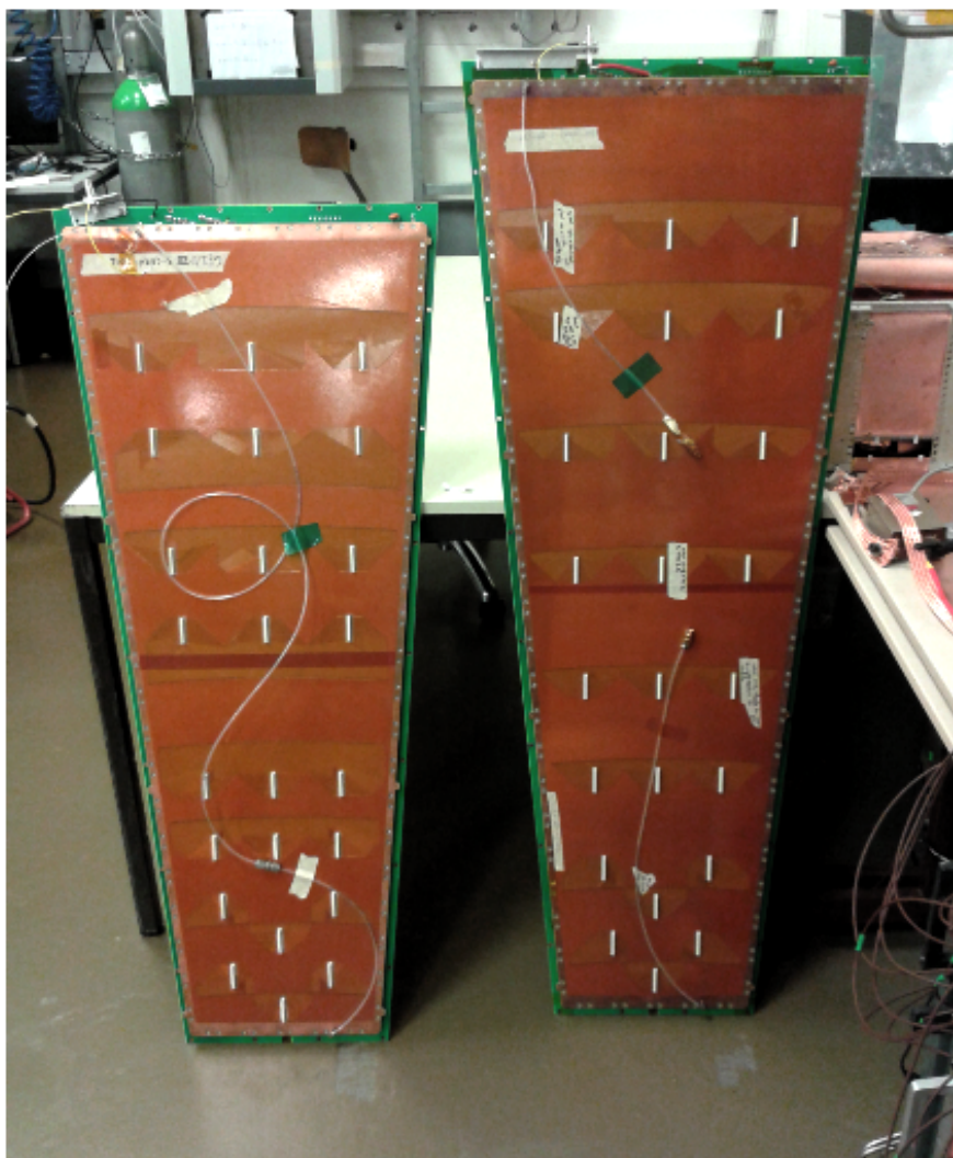
Figure 4.14: Short and long triple-GEM chambers assembled for the slice test of CMS.
