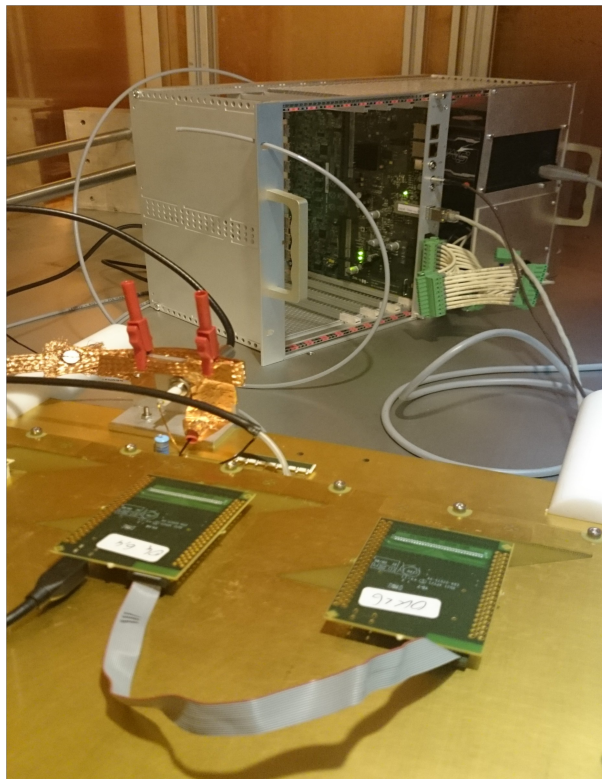
Figure 5.56: The first gain uniformity test with 30cm x 30cm triple-GEM prototype at Gent university laboratory.
