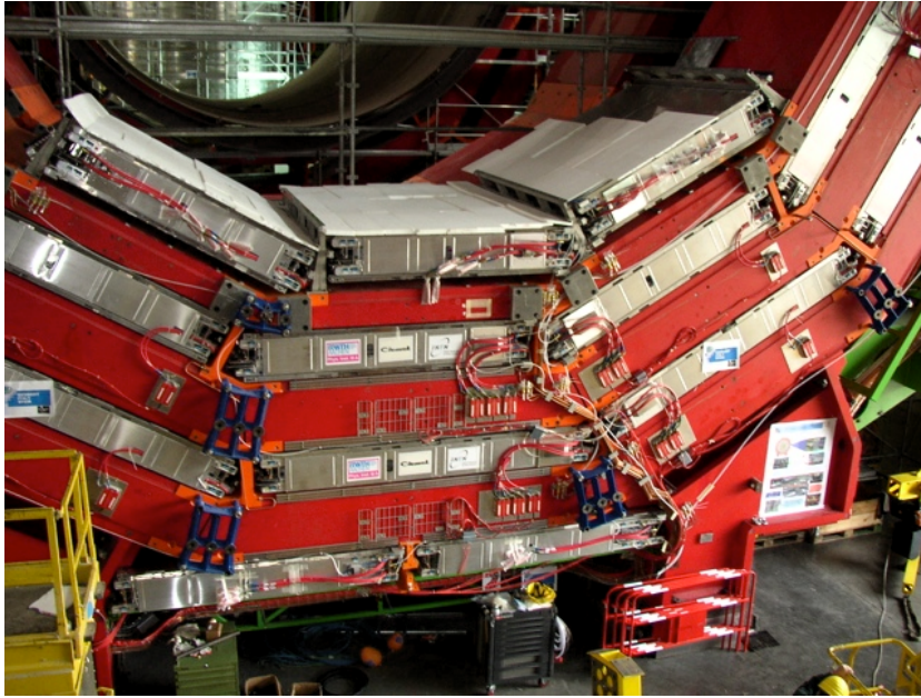
Figure 4.1: The DT region in the CMS muon system
