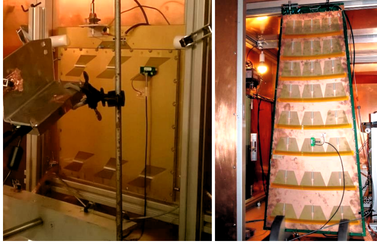
Figure 5.50: 30cm x 30 cm small prototype and GE1/1-IV chamber at Ghent University CMS-GEM laboratory.
