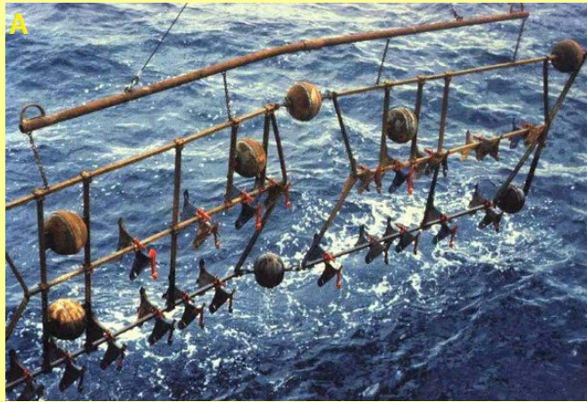
Figure 1-15. Picture of the plough-harrow with double-sided plow shares that was used to disturb the sediment of the DEA. Source: https://www.discol.de (accessed: April 1 st 2018).
