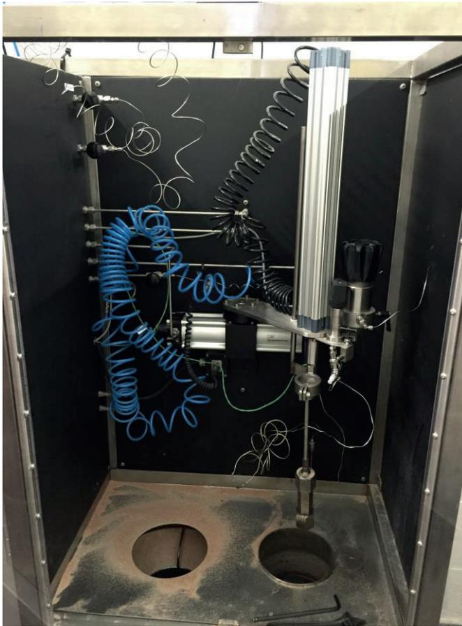
Figure 2-4 Picture of the batch reactor
