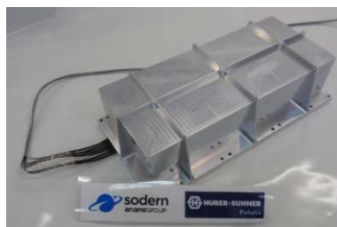
Figure 4-3 Picture of the Optima 48-port switch breadboard
