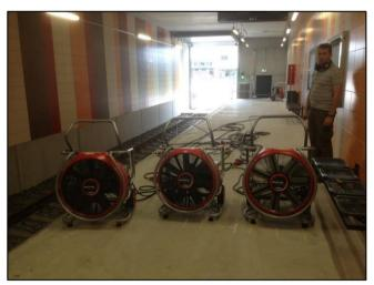
**Figure 7** Three fans placed on the platform in the Frankfurt subway building. The fans are positioned with reference to the centre line of the stairs. From right to left: -25cm, +67cm and +150cm. The stairs are behind the photographer. The fan on the right in the picture is addressed as 'left' in the text and vice versa.
