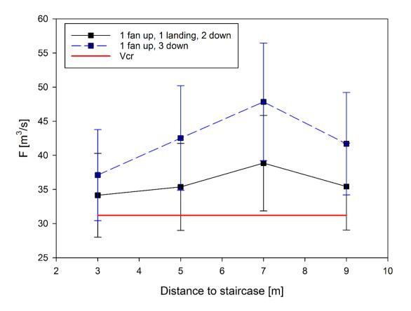
**Figure 10** Flow generated by four fans: Comparison of two different types of set ups. One type A fan was placed at the exit door of the building. Two type B fans were placed on the platform. The third type B fan was placed on the landing in test 68-71 (solid line) or on the platform between the two other fans in test 72-75 (dashed line). The red line indicates the flow rate corresponding with the critical velocity.
