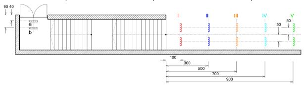
**Figure 3** Position of the three fans during tests 29 through 38. Two different positions were used at the top of the staircase. The fan in position 'a' was placed 40 cm from the exit in tests 29 through 33. Position 'b' is 90 cm from the exit. This position was used during tests 34 through 38. These positions were combined with 5 positions (I to V) on the platform, ranging from 1 m to 9 m from the stairs. This combination leads to 10 experiments.
