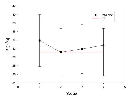
**Figure 6** Influence of top position: Comparison of 4 positions at the top of the staircase (tests 56 – 59): from left to right: 40 cm, 90 cm, turn close and turn far. The positions of the fan are found in Figure 5. The red line indicates the flow rate corresponding to the critical velocity.
