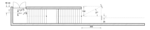
**Figure 5** Four different fan positions at the top of the staircase. Position a: 40 cm from the door during test 56. Position b: 90 cm from the door during test 57. Position c: 40 cm from the door on the line that connects the centre of the door with the centre of the stairs ('turn close') during test 58. Position d: 90 cm from the door on the line ('turn far') during test 59. Two additional fans were placed on the platform.
