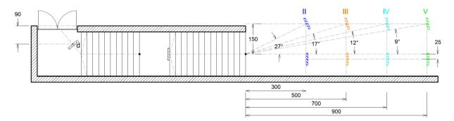
**Figure 9** The set-up of experiments 68 to 71 and 85-88. The type A fan upstairs was in the 'turn far' position. On the landing, there was 1 type B fan. The two fans on the platform were placed at 4 different distances. The inclination of the fans was 10°. In experiments 89-92, the same set-up was used but the inclination of the fans on the landing and platform was changed to 18°.
