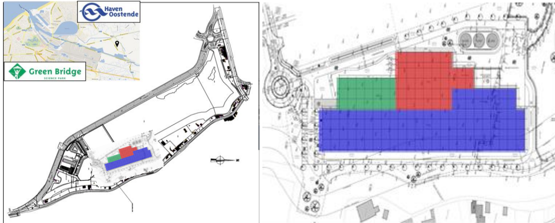
Figure 2. Top - Location of the upcoming physical modelling research cluster near the port of the Ostend. Bottom - red upper right part: COB main hall, blue lower part: towing tank, green upper left part: shared office space.
