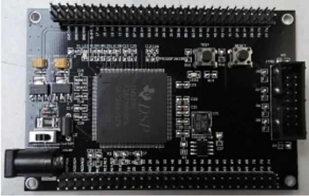
Fig. 3. TMS320F28335 system development kit.
