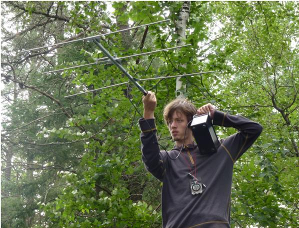
**Figure 2.3:** A researcher picking up the radio signals of VHF transmitters (Source: [lesnoezero.villagepages.org](http://lesnoezero.villagepages.org)).
