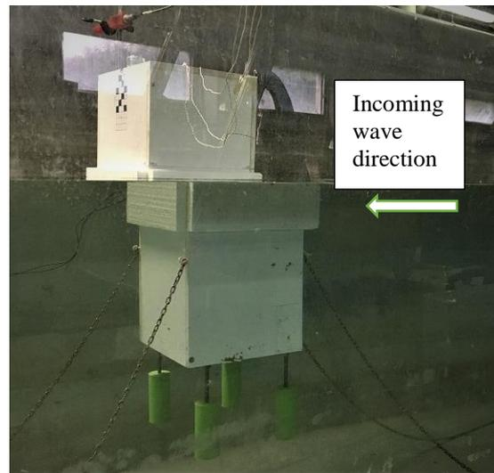
Figure 6. Side view of the mooring system.
