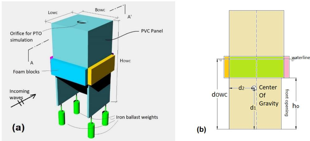
Figure 1. Geometry of the OWC WEC model: (a) 3D Sketch. (b) Cross-section A'A'.
