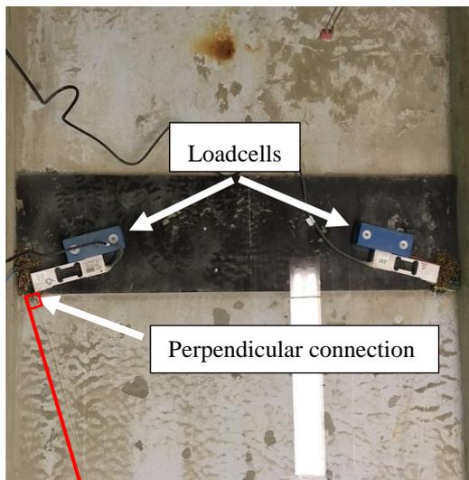
Figure 5. Load cells configuration on top view.
