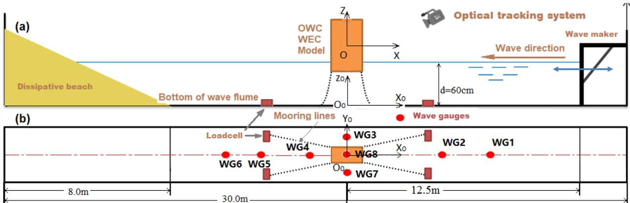
Figure 2. Side view (a) and top view (b) of the experimental layout.
