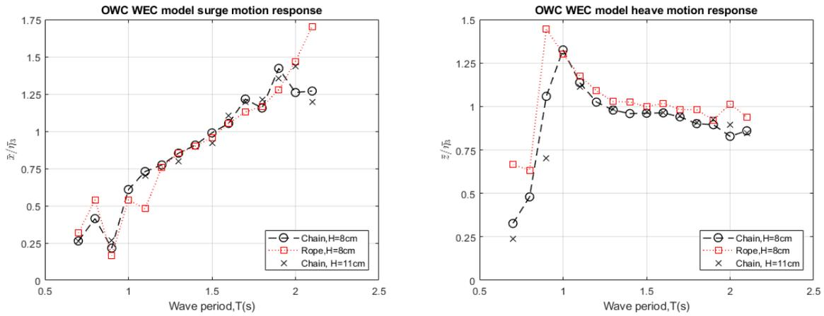
Figure 8 OWC WEC model surge (left) and heave (right) motion amplitude response in small amplitude waves.
