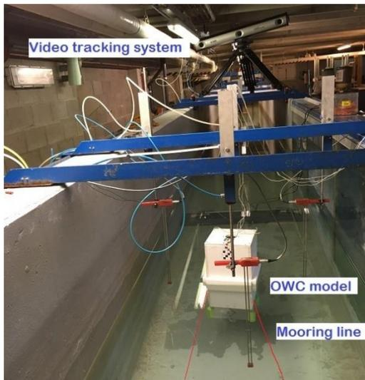
Figure 3. Optical motion tracking system.
