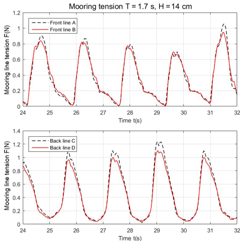
**Figure 10 Mooring line horizontal tension measured at the anchor point.**
