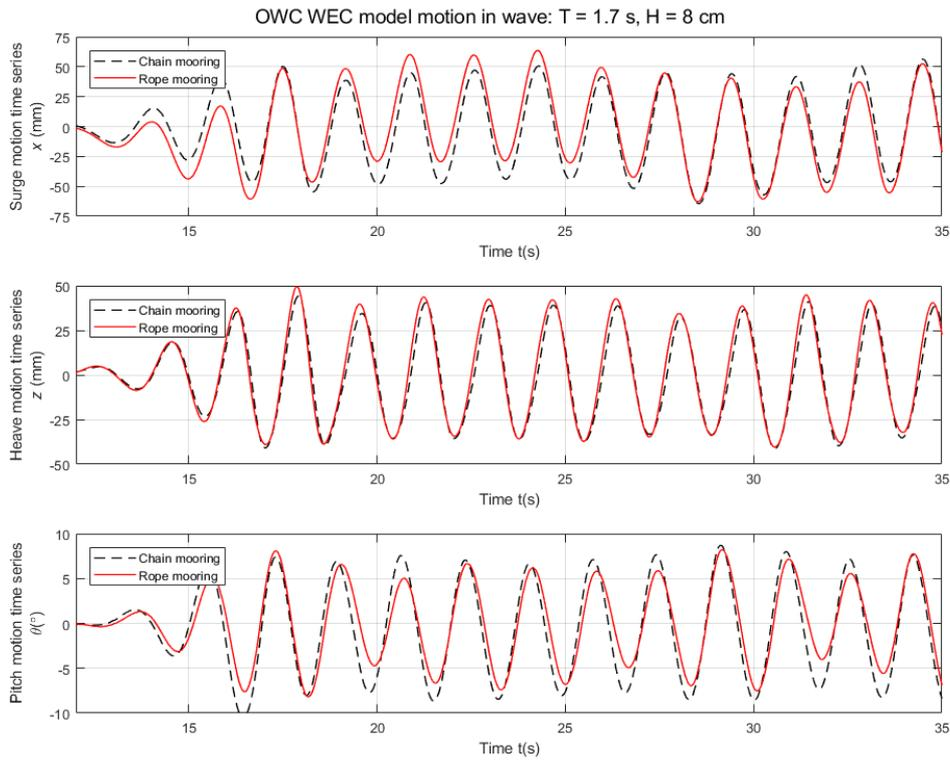
Figure 7 Surge and heave motion response in small amplitude waves.
