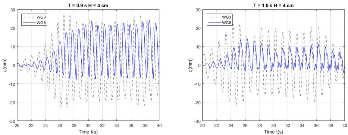
Figure 9 Comparison between water column surface elevation inside OWC WEC chamber (WG3) and external wave surface elevation (WG8) near heave resonance zone  $T = 0.9$  s (left) and  $T = 1.0$  s (right).
