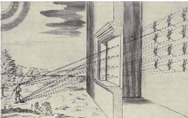
(fig. 2) Illustration of a camera obscura building with 12 apertures, published in Bettini's Apiaria universae philosophiae mathematicae , 1642.
