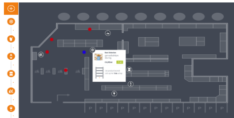
Fig. 5. Printscreen of the smart shopping cart application with the shopping list products positioned on the supermarket map. When the shopping cart (blue dot) gets nearby a product, more information is provided on the price, number and shelf position of the product.
