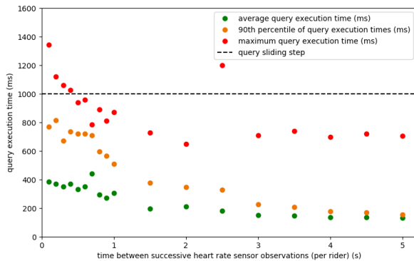
Figure 6: Query execution times for varying time between successive heart rate observations per rider, for 5 riders. Query window size is 10 seconds, sliding step is 1 second.
