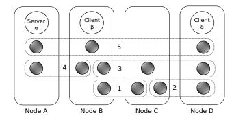
Fig. 1. A simple example of RINA layering. Scope for layers 1, 2 and 4 is local to a physical link. Scope for layers 3 and 5 is larger and spans multiple nodes.
