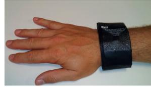
Fig. 7. Designed textile coil embedded in a leathered bracelet.
