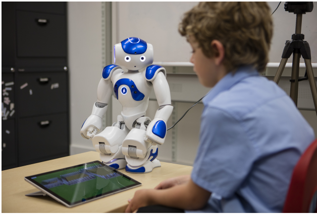
Fig. 1 The L2TOR setup includes the NAO robot standing to the side of the child with a tablet in between them.
