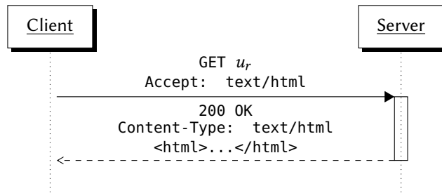
Figure 2.1: A client requests a resource identified by URL u_r in a HTML representation using HTTP. The server responds successfully with the HTML page.
