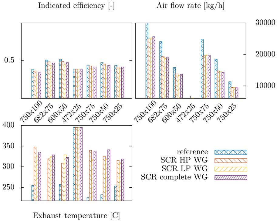
Figure .6: Wastegate configuration simulation: efficiency, airflow rate and exhaust temperature as a function of [engine speed x engine load]
