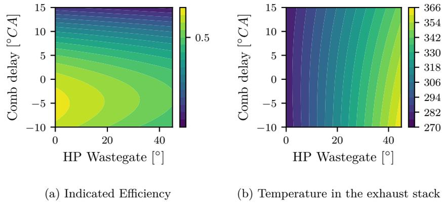
Figure .5: Simulation results as a function of complete wastegate position and combustion delay.
