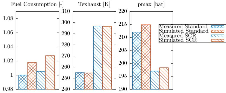
Figure .9: Simulation compared to measurement at full load, for lowest fuel consumption and increased exhaust temperature
