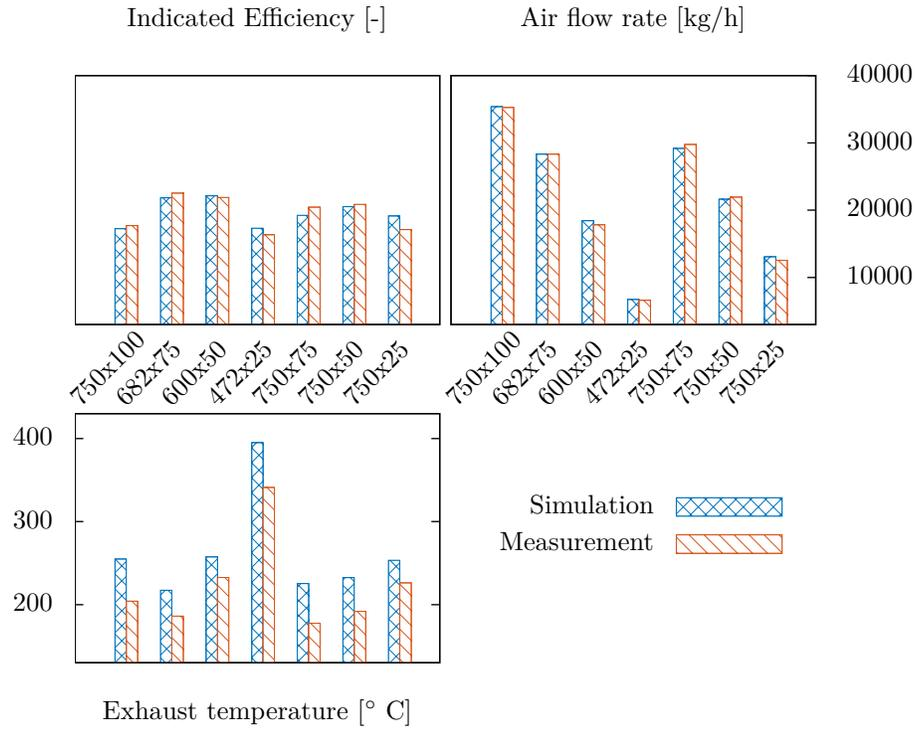
Figure .2: Validation of the simulation code: efficiency, airflow rate and exhaust temperature as a function of [engine speed x engine load]
