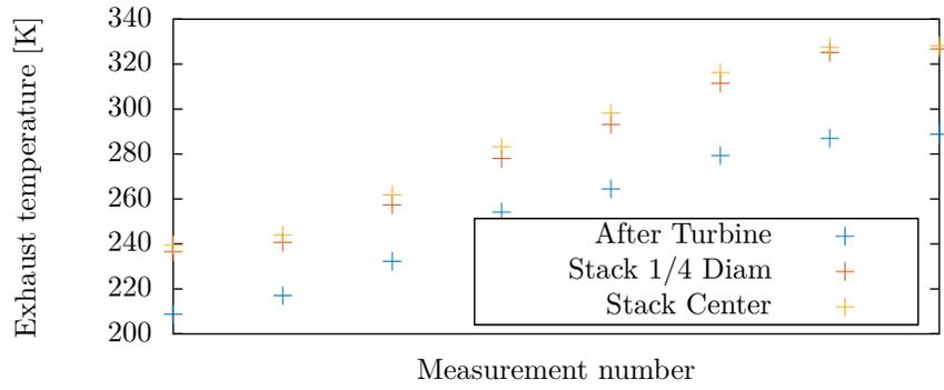
Figure .3: Sensor position (after turbine, and two positions in exhaust stack) influences measured temperature, measurements with variable wastegate position.
