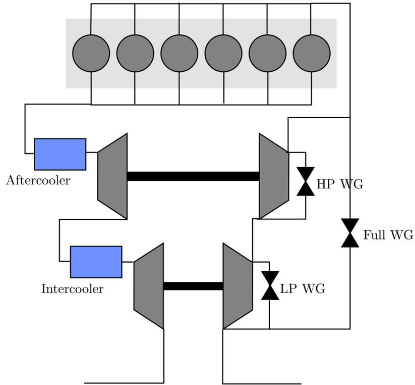
Figure .1: Schematic view on engine gas path with High Pressure Wastegate (HP WG), Low Pressure Wastegate (LP WG) and Full Wastegate (Full WG)
