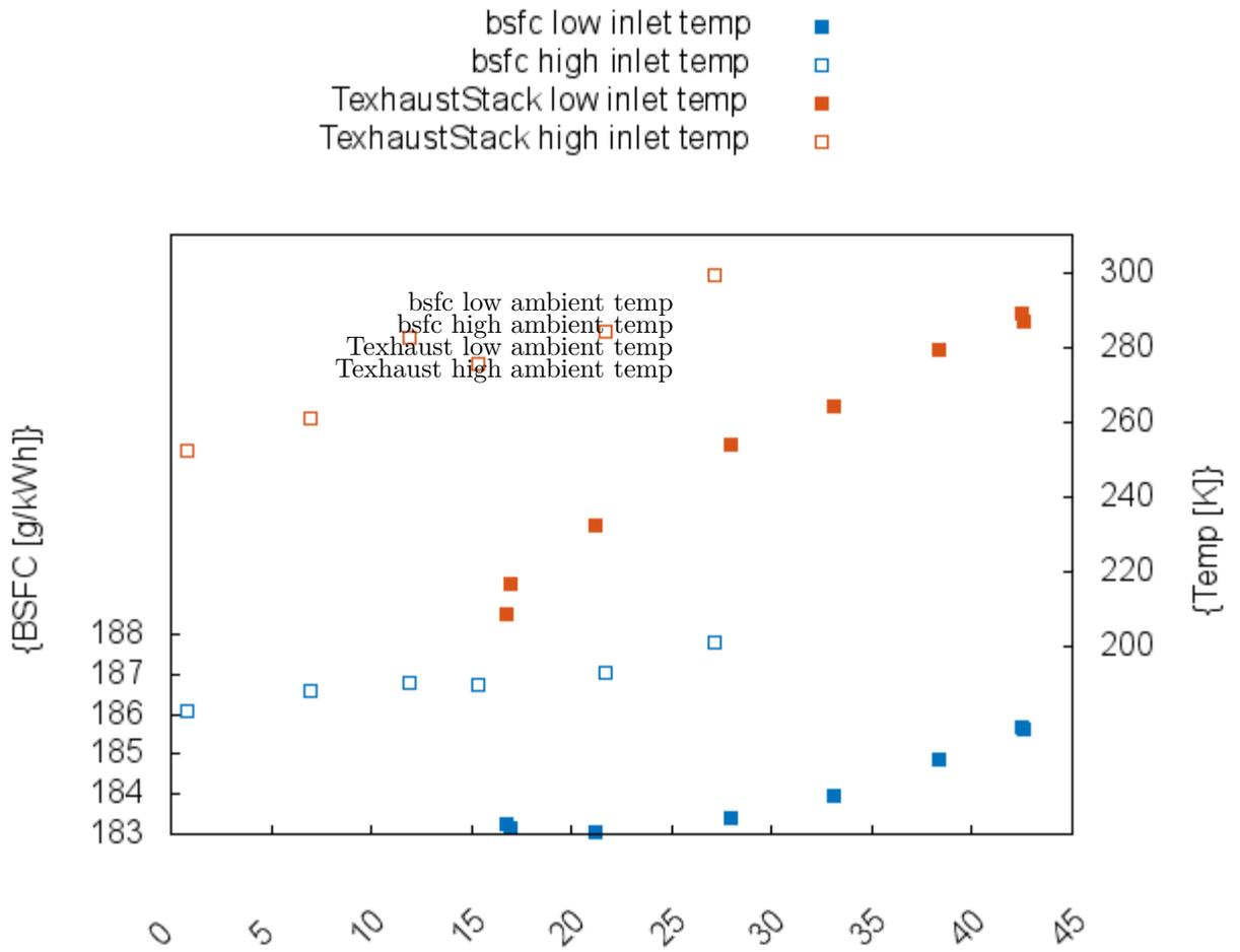
Figure .8: Specific fuel consumption (blue) and exhaust temperature (red) as a function of wastegate position at full load during engine measurements
