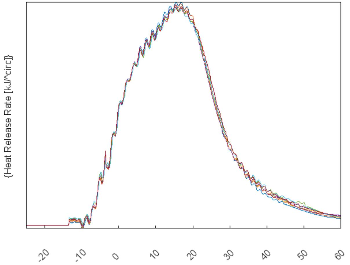
Figure .7: Heat release rates with wastegate position varied between 0° and 45°.
