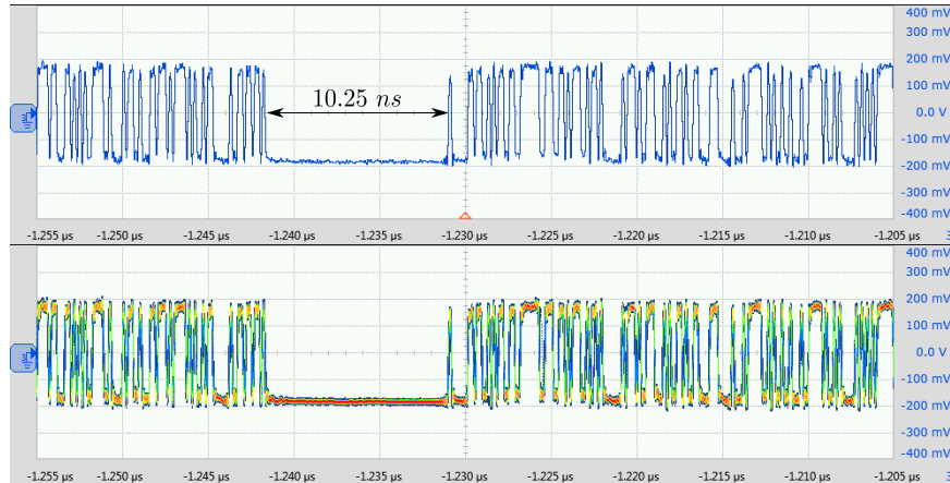
Figure 6.24: A packet in optical burst mode measurements with a short gap ( 10.25\text{ ns} ).
