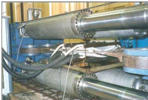
Figure 6: Cooled CWP specimen mounted in the 8000 KN load frame ready for tensile testing.
