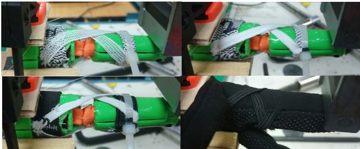
Figure 3. Four prototypes: A01 (top left) and A02 (top right) have inelastic cruciate ligaments A03 (bottom left) and A04 (bottom right) have elastic cruciate ligaments
