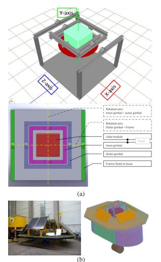
Figure 4: (a) CAD drawing of stabilization mechanism, (b) 3E working prototype and FE model
