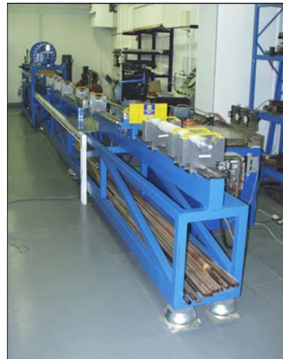
Fig. 2. Split Hopkinson tensile bar setup of DyMaLab of Ghent University.
