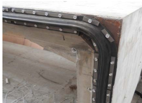
Figure 7 Detailed view of model rubber seal after installation
