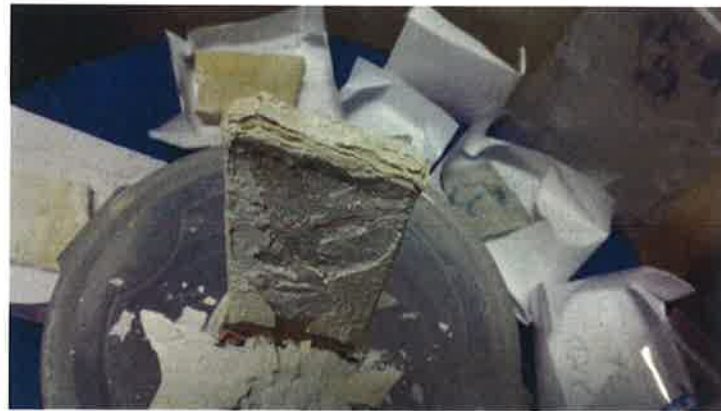
Figure 5: Visual observation of reacted CSA paste specimen partially immersed in \text{Na}_2\text{CO}_3 for 10 days
