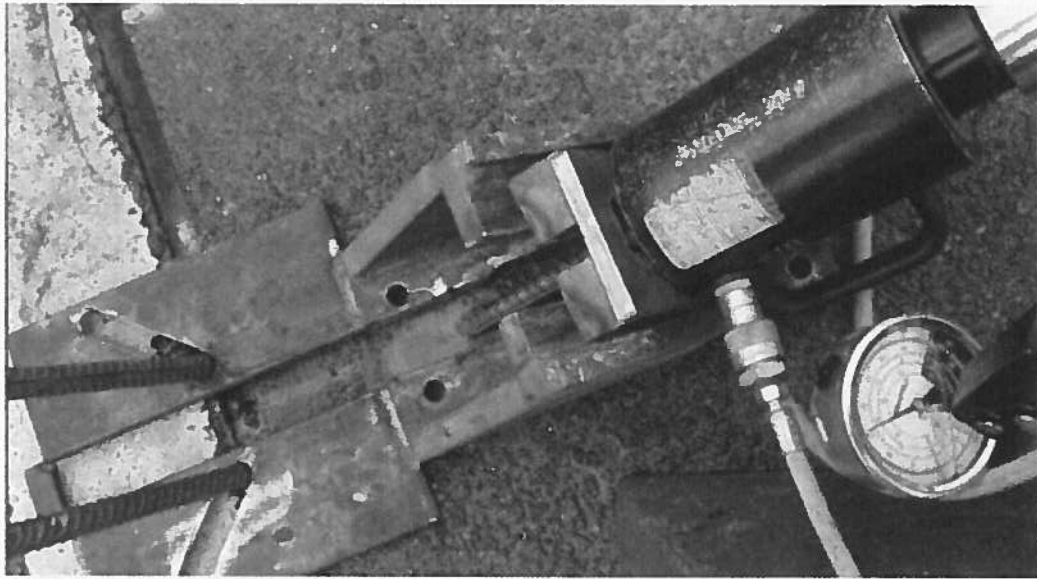
Figure 10. Tensile test on a elongated tie bar on site
