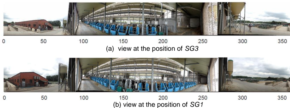
Figure 43: View with surrounding obstacles for (a) SG3 and (b) SG1, projected on a scale of degrees referring to the wind direction
