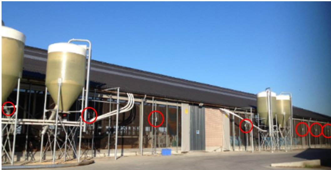
Figure 38: Photo of the NE -side of the dairy barn with anemometers on a horizontal line (marked with red circles), equally spaced over the openings
