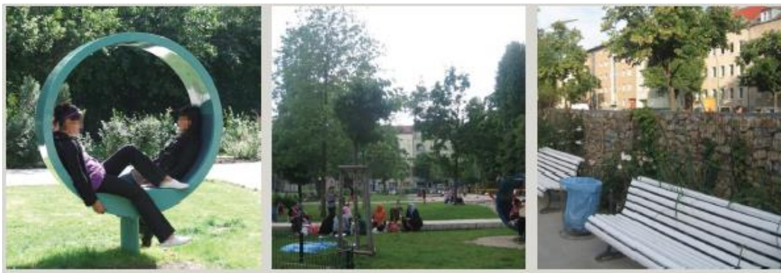
Figure 7 - Example of the soundscape intervention in Nauener Platz, Berlin (Germany), using a gabion wall (right) to protect park goers from noise around the playground area; audio islands (left and centre) were also installed to provide areas of restoration
