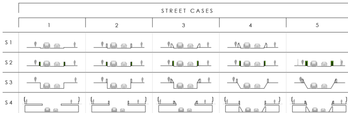
Figure 2–Street configuration cases (S). Sequences are distributed horizontally. S1 Low barrier shape. S2 Green absorption on low barrier. S3 Depressed road. S4 Two level street.
