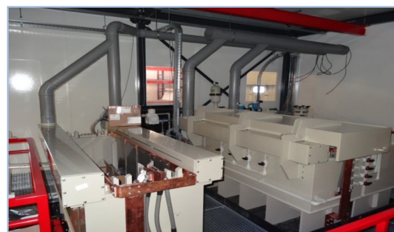
Fig. 2: Due to the promising features of this new electrodeposition solvent, a flexible semi-industrial pilot plant has been designed in OCAS NV. In this way, several set-ups, IL compositions, additives, etc. can be tested and evaluated on a large scale, and compared with lab scale experiments.
