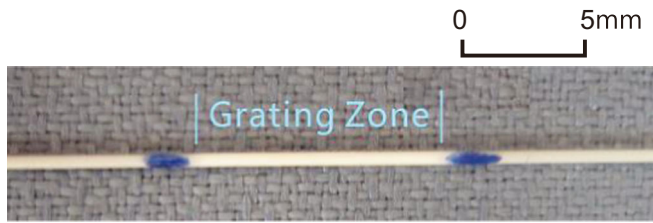
Fig. 8 Encapsulated FBG sensing fiber
