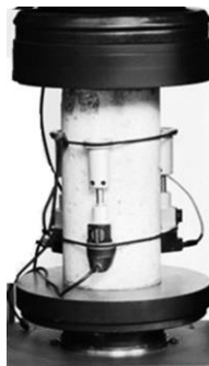
Fig. 5.3 Example of a static E modulus measurement set-up with stress-strain gauges fixed on the sample, which is placed in compressive strength test cell. Figure adapted from Controlsgroup.
