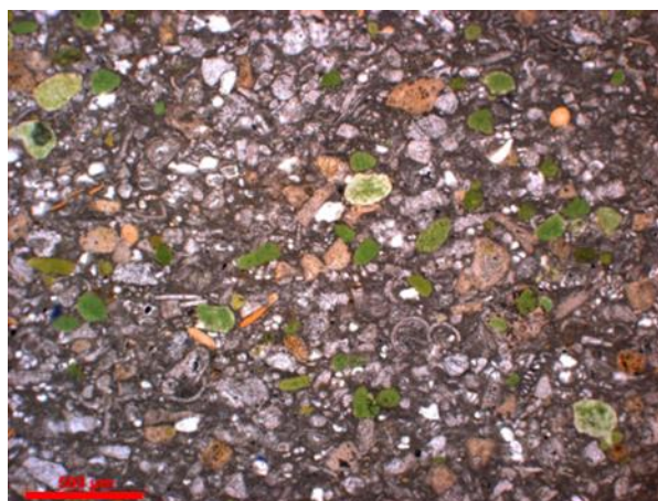
Fig. A7.2 Microscopic view of the stone from the Couvent des Ursulines, Mons, in plane polarized light. The scale bar represents 500 \mu\text{m} . A matrix of micrite is present, surrounded by bioclasts such as foraminifers, large glauconite and phosphate grains and some angular quartz.
