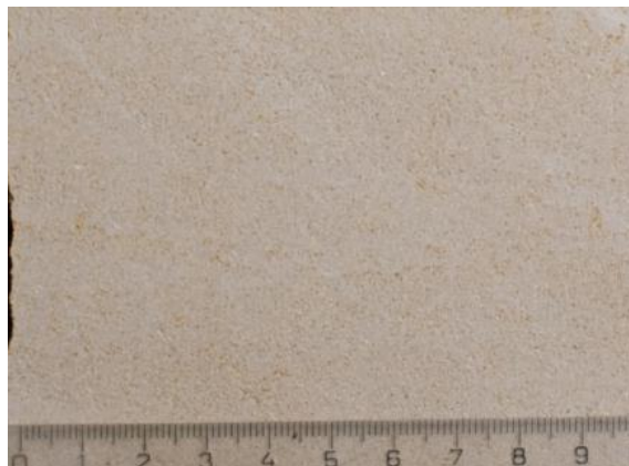
Fig. 7.4. Macroscopic photo of the Savonnières limestone used in this study. The scale is in centimetre.
