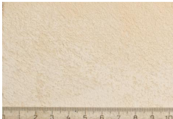
Fig. 7.2 A macroscopic image of the sawn surface of the Maastrichter stone sample used in this study. The scale is in centimetre.
