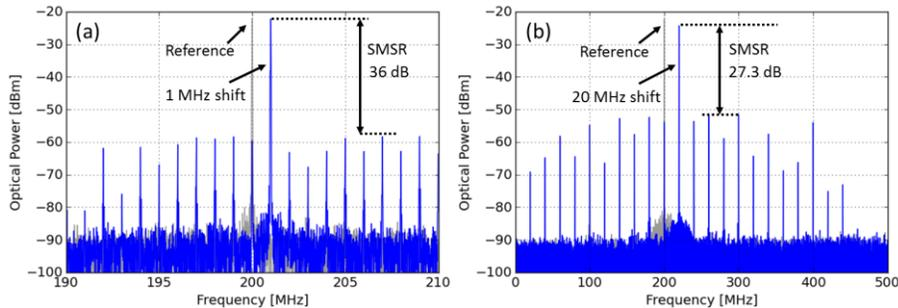
Figure 2: Measured electrical spectra with (blue) and without (grey) additional frequency shift in case of (a) a 1 MHz shift with a triangular drive signal and (b) a 20 MHz shift with a sinusoidal drive signal.
