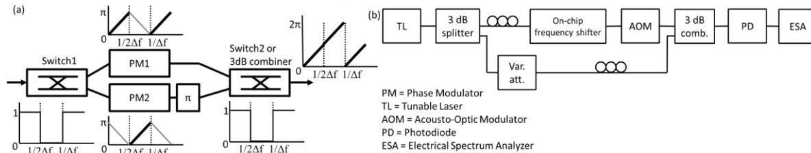
Figure 1: (a) Schematic overview showing the working principle of the proposed frequency shifter. (b) Schematic representation of the measurement setup.
