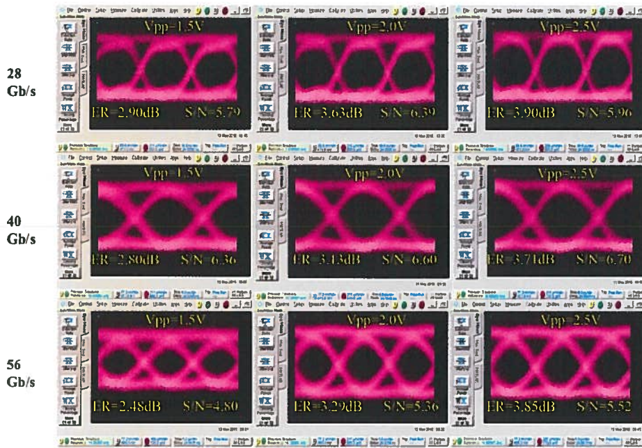
Fig. 7. Measured eye diagrams at room temperature at 1610 nm with 1.5 V pp , 2.0 V pp and 2.5 V pp swing and with data rates of 28 Gb/s, 40 Gb/s and 56 Gb/s with input power of 0 dBm.
