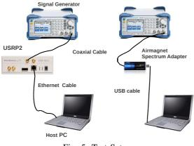
Fig. 5: Test Setup
