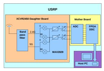
Fig. 1: USRP Block Diagram
