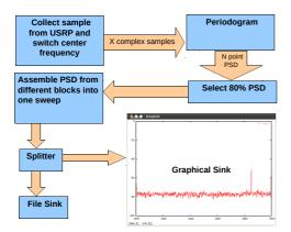
Fig. 3: Iris Component Diagram
