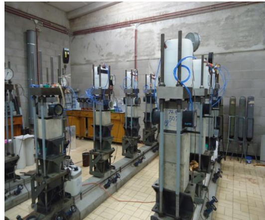
Figure 1. Chloride and load combined attack setup (Splitting)
