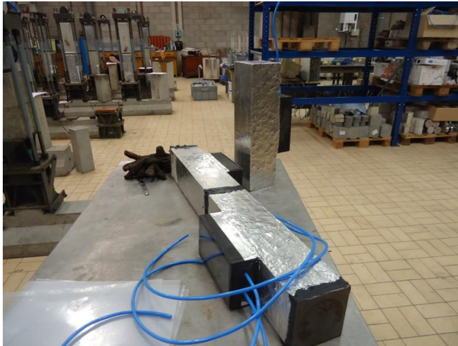
Figure 2. Chloride and load combined attack setup (compression)
