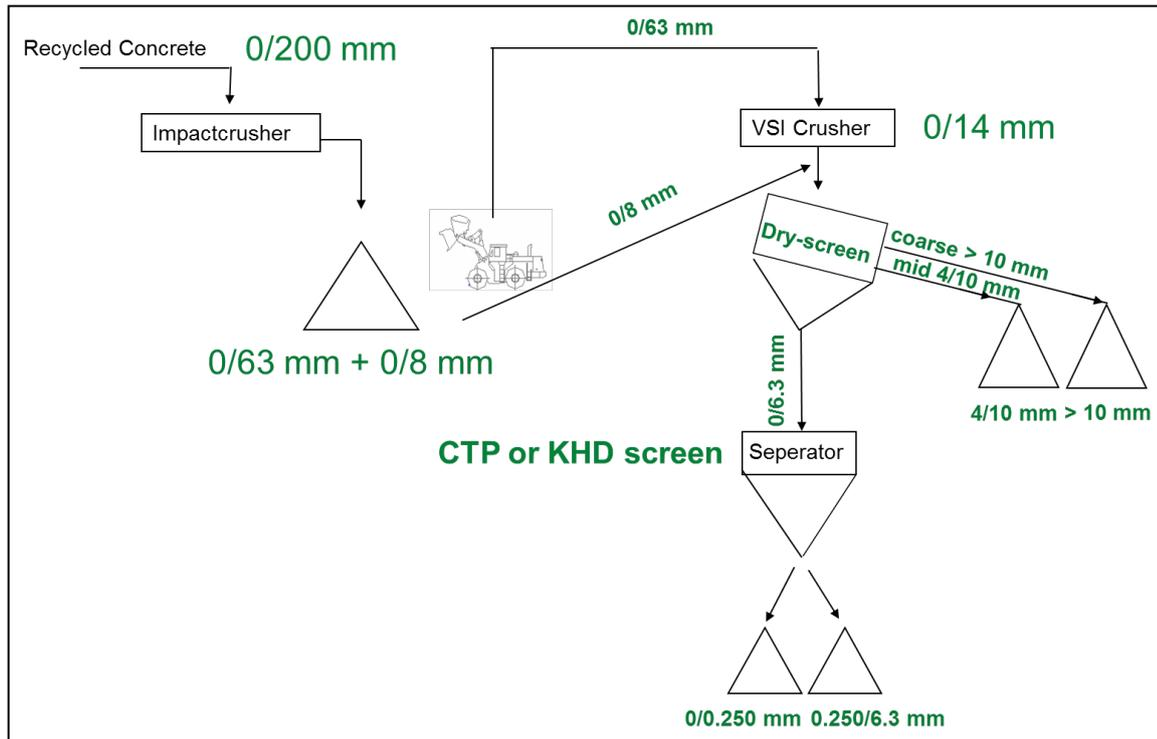
Figure 2 – Process view incorporating the CTP and KHD separation
