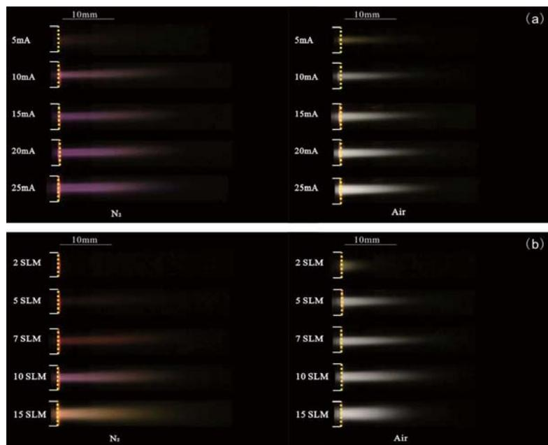
Figure 4.5: Photographs of the afterglow of the DC plasma jet under different conditions: (a)  $N_2$  and air discharge at various discharge currents; (b)  $N_2$  and air discharge at various gas flow rates.
