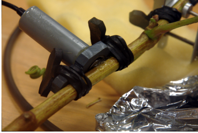
Figure 4.1 The point-contact sensor was installed normal to the branch surface using a custom-made PVC holder with spring inside. Photo credit: Sim Minnaert
