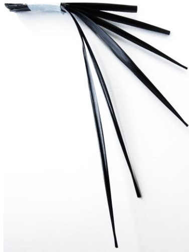
Figure 3 Cured geometry of cantilevered M18/M55J prepreg samples
