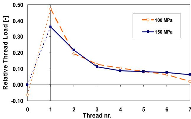
Fig. 9: Thread load distribution (numbering as in Fig. 3)
