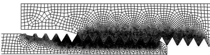
Fig. 4: Mesh of the FE model
