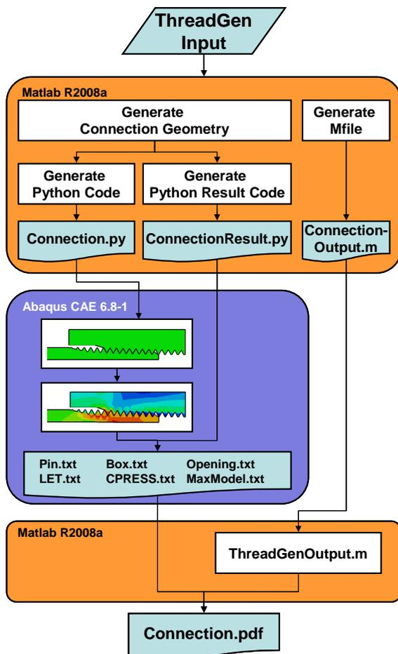
Fig. 1: Structure of the parametric program *ThreadGen*®
