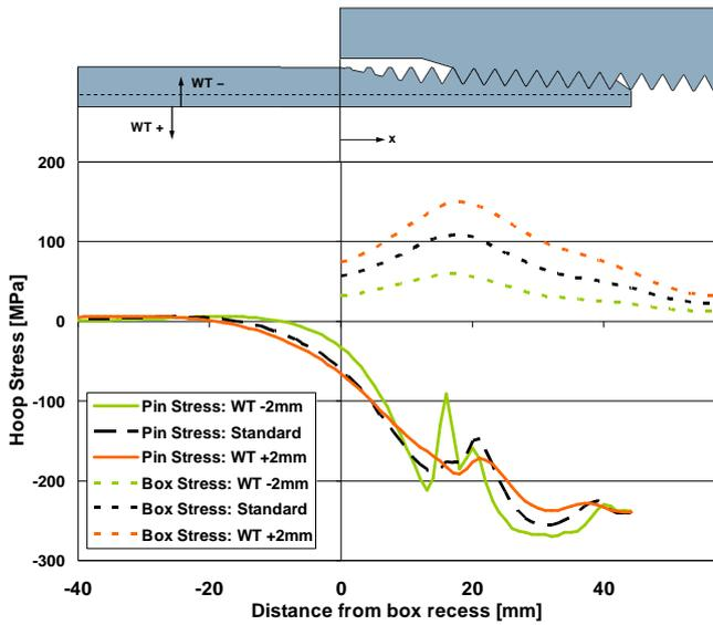
Fig. 14: Hoop stress at the inside wall of the pin and the outside wall of the box at make-up for different values for the pin wall thickness.
