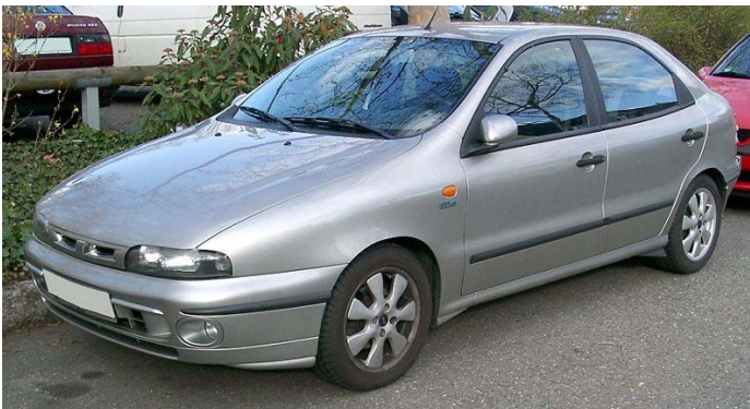
Fig 2. 'average' car approx 1300kg total, drag coefficient 0.3; 2m 2 cross section.
