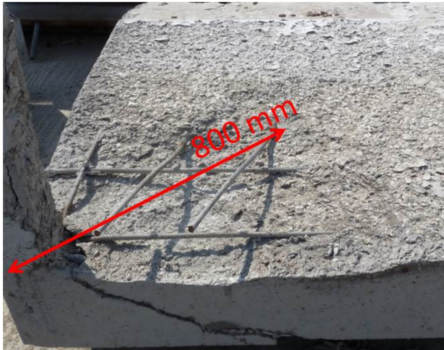
Fig. 11 Spalling damage of slab S0
