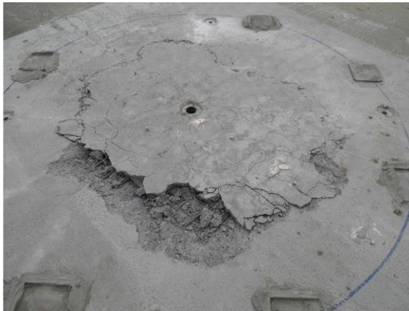
Fig. 7 Punching cone after fire test of slab S1 (top view)
