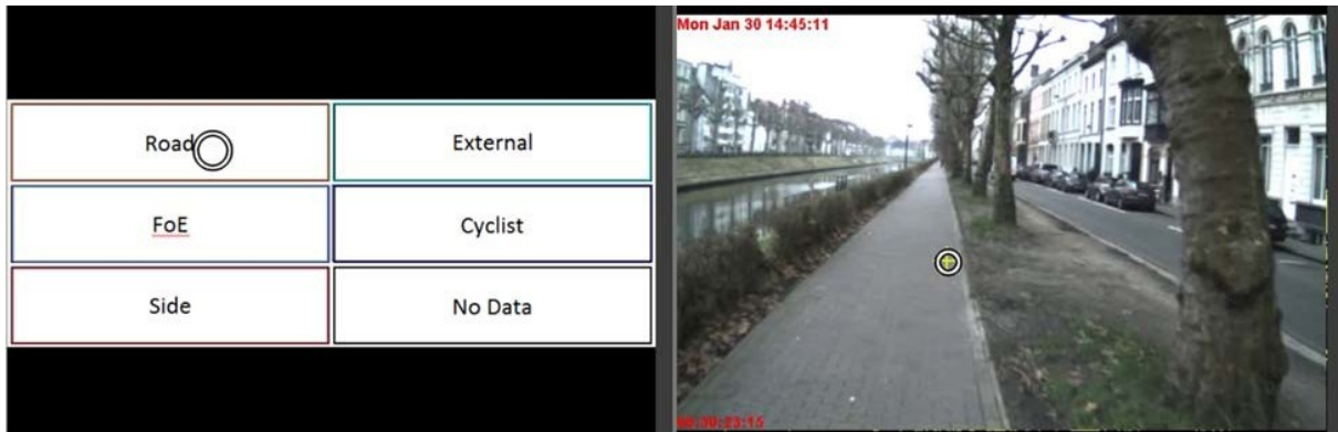
Figure 4 : Example of fixation-based procedure: at the right the video is shown with fixation marker, at the left six possible AOIs are shown to which the fixations can be assigned (print screen of BeGaze 3.2).
