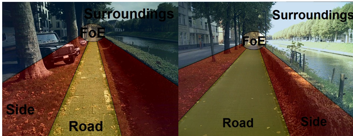
Figure 2 : Screen shot of the Low quality (left) and high quality (right) cycling track with AOI overlay. Note that this grid was not used to determine the fixation location, each of the fixations was assigned manually to one of these AOIs, or to a fifth AOI 'Pedestrians & cyclist'.
