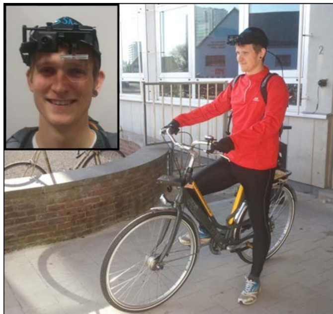
Figure 1 : Participant on bicycle wearing the head-mounted eye-tracking device (SMI). Inset: frontal view of eye tracker
