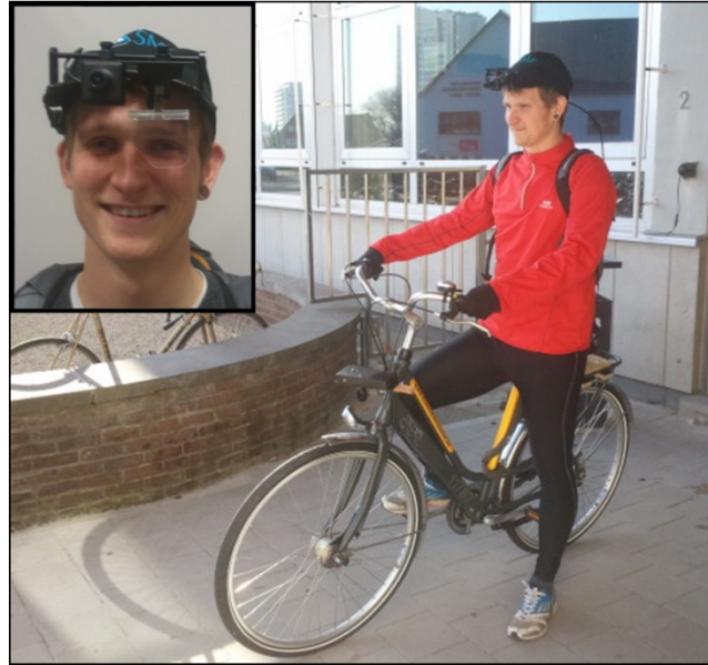
Figure 1 : Participant wearing on bicycle wearing the Head-mounted Eye-tracking Device (SMI). Insert: frontal view of eye tracker.
