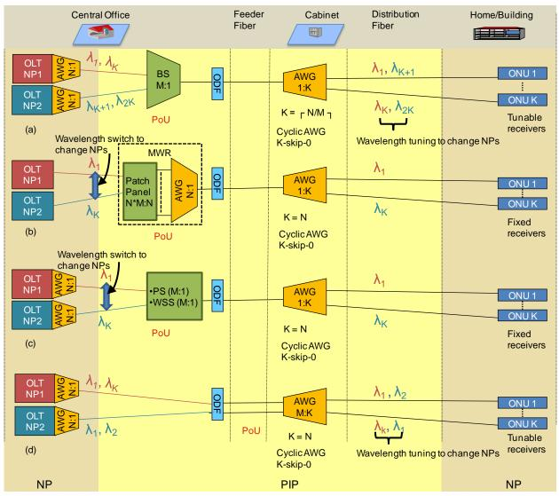
Figure 3: Wavelength Open access schemes at the OLT interface for WDM-PON with point of unbundling (PoU) as: a) BS b) MWR c) PS/WSS d) FF. Wavelength mapping shows how OLT connects with ONU1 and ONUK and N = number of wavelengths; M= number of NPs; K = number of users.
