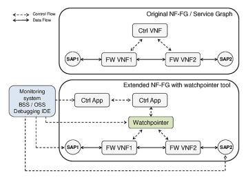
Figure 4: Use case over a watch-point inserted for observing data plane and control messages.
