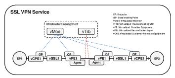
Figure 3: Simplified graphical representation of SSL VPN.
